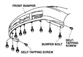
7. Install a self-tapping screw through each spring nut.
