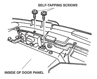
Inside the door panel, press the retaining tab with a flat-tip screwdriver, and raise the remote control door mirror switch.
