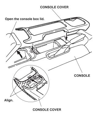
12. Thoroughly clean the bonding surfaces where the console cover will attach; remove the adhesive backing from the console cover, and attach the cover to the console by pressing firmly with the palms of both hands. Remove the masking tape.
