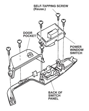
Position the power window switch and the door pocket you just removed onto the new left door switch panel from the kit, and reinstall the six self-tapping screws.
