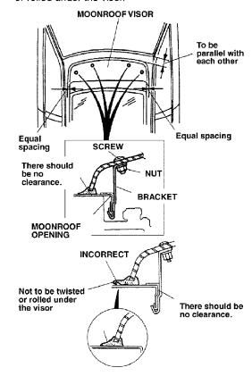
Tighten the nuts and screws, alternating between sides. To prevent damage to the resin nuts, do not overtighten the screws.
