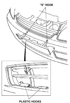
11. Snap the nose mask to the snap-screw. Repeat on the other side of the vehicle.
