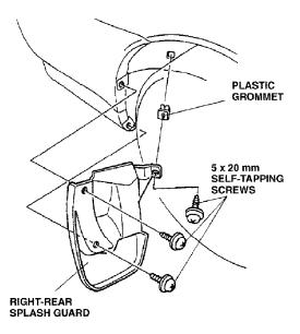
Position the right-rear splash guard on the rear bumper, and install three of the 5 x 20 mm self-tapping screws supplied.
