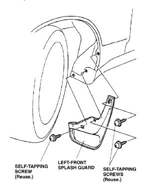
Turn the steering wheel all the way clockwise, and repeat steps 3 and 4 to install the right-front splash quard.
