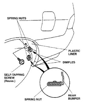
Position the left-rear splash guard on the rear bumper, and install two of the 5 x 20 mm self-tapping screws supplied and the self-tapping screw removed in step 6.
