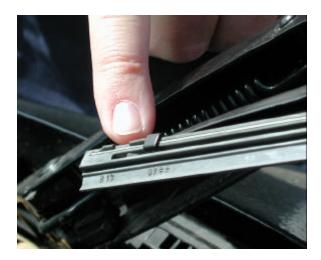
12. Blade will stop sliding near the end. where the locking notch is.
