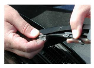
10. Slide insert through notches at bottom of wiper blade.
