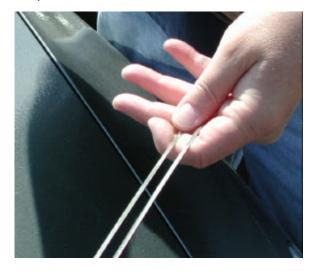
6. Discard rubber blade material and keep the two reinforcing strips
