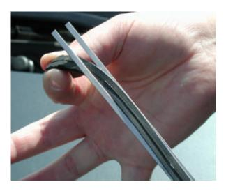
5. With insert completely removed from the wiper arm separate reinforcing strips from rubber material
