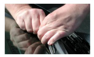
3. Hold wiper arm with one hand and pull out on insert.
