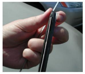
7. Slide reinforcing strips into new wiper insert as shown
