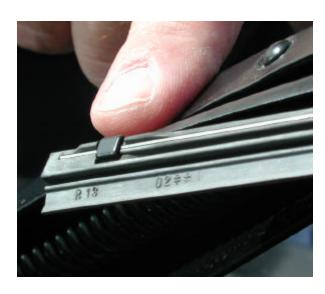
14. Insert is secured when notch on wiper arm is between the two raised areas on the insert.
