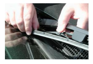
4. Once wiper insert releases from bottom of wiper arm slide insert out assembly
