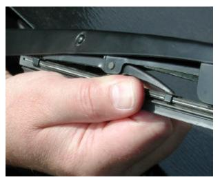
13. Apply pressure to insert to pull it past the first notch.
